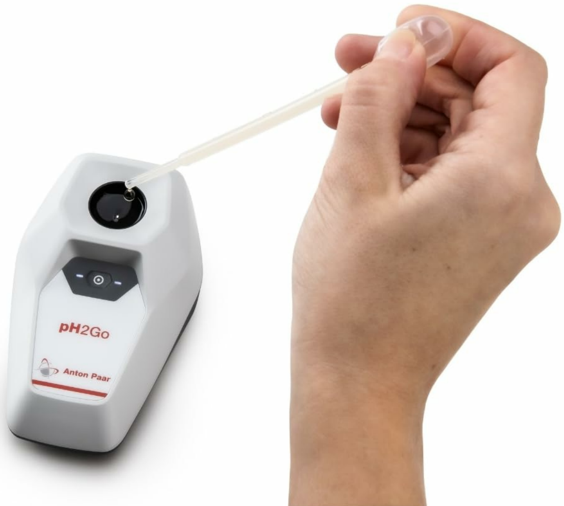
Figure 4: Applying a 0.5 mL sample to the pH2Go. This image demonstrates the precise application of a small liquid sample into the pH2Go's sensor well using a pipette.
