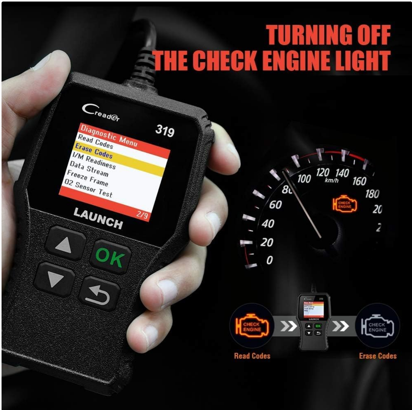
Image: The CR319 displaying "Erase Codes" on its screen, with an illustration showing the process of reading codes, then erasing them to turn off the Check Engine Light on the vehicle's dashboard.
