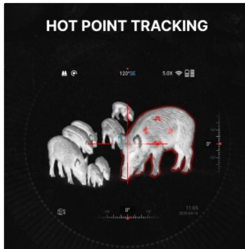
An image demonstrating Hot Point Tracking, where the warmest object (a wild boar) is highlighted.
