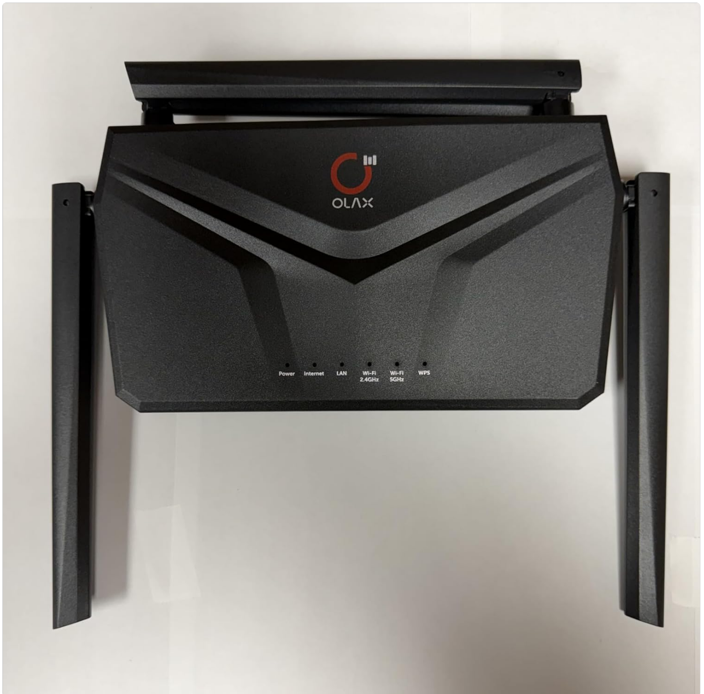
Image: Front view of the OLAX Scorpio X60 Router, showing LED indicators for Power, Internet, LAN, Wi-Fi 2.4GHz, Wi-Fi 5GHz, and WPS.
