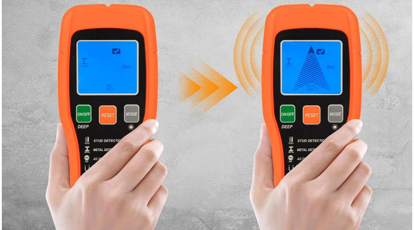
Figure 3: The wall scanner in Metal Scan mode, showing detection of rebar within a wall. The display indicates increasing signal strength as the device approaches the metal object.
