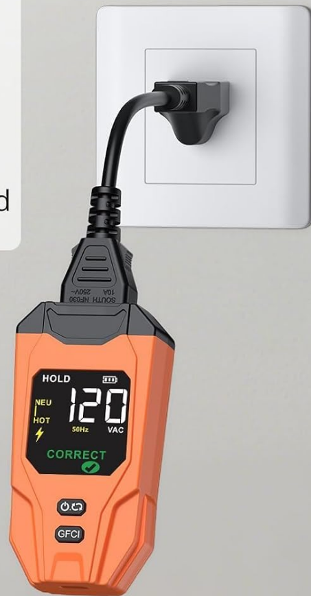
Image: The transmitter's display showing different detected wiring states for an electrical outlet.
