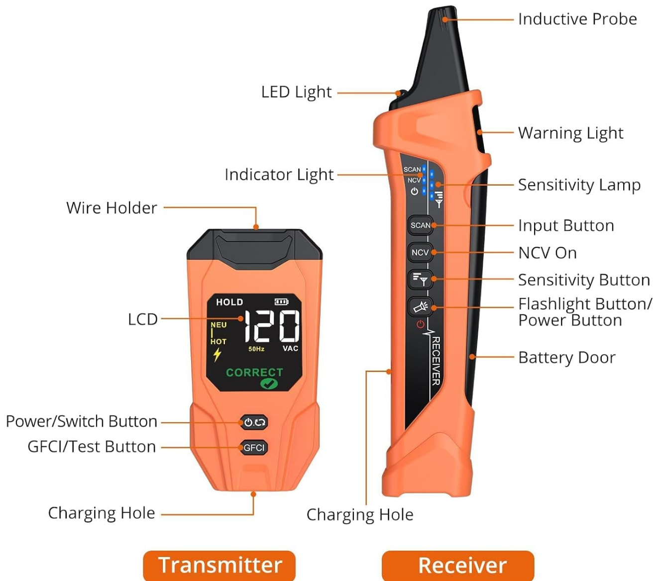
Image: Labeled diagram of the transmitter and receiver components.
