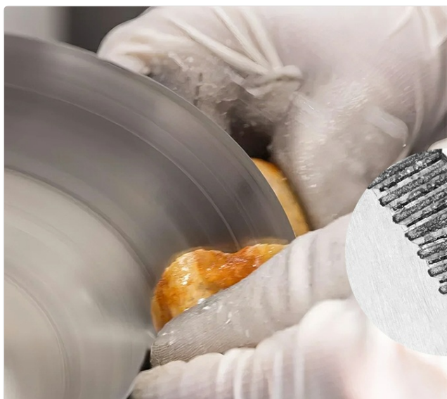
Figure 5.1: Cutting a rock with the diamond saw blade.
