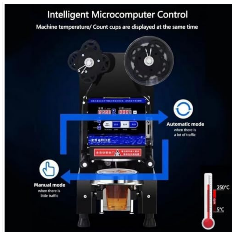
Figure 3: Control panel with options for automatic and manual operation. Temperature and cup count are displayed.
