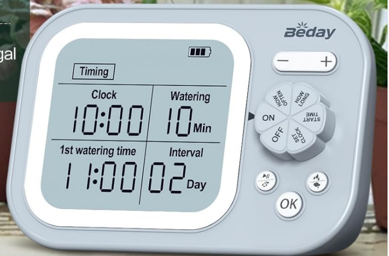
Figure 3: Example of the timed automatic watering display, showing programmed settings for watering duration and interval.
