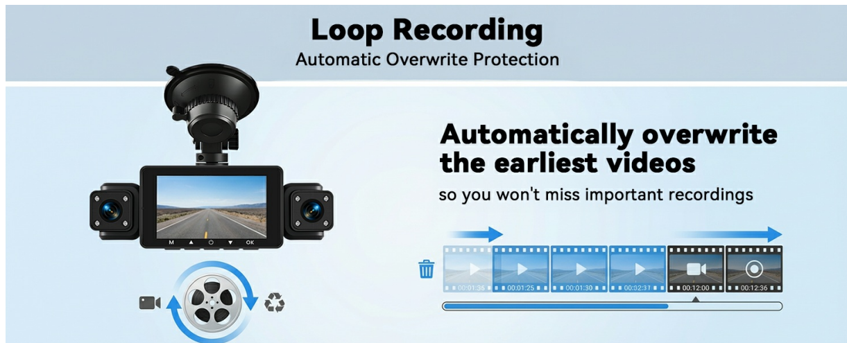
Figure 6.2: Loop Recording mechanism.
