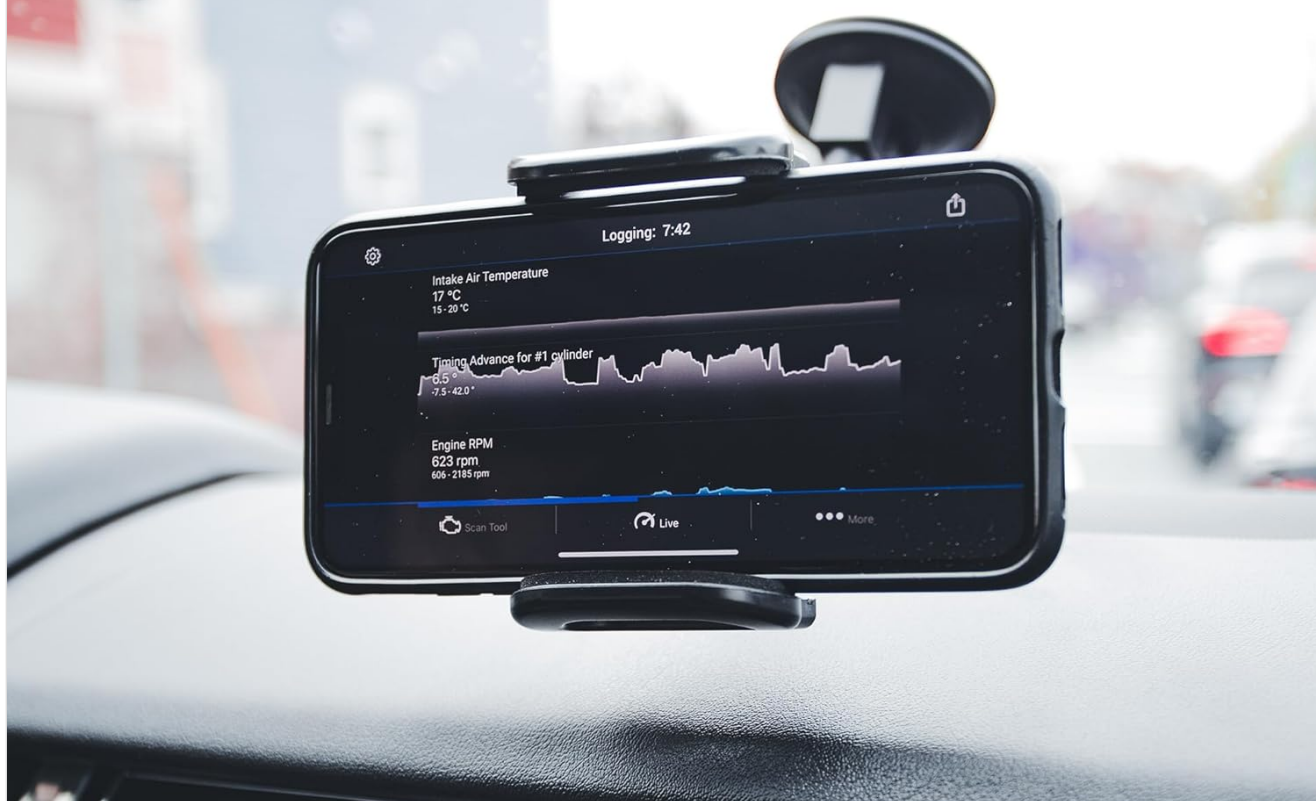
Image: A smartphone screen showing live vehicle data, such as intake air temperature and engine RPM, mounted in a car.
