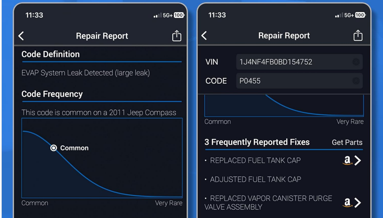
Image: An example of a repair report within the BlueDriver app, detailing a code definition and suggested fixes.
