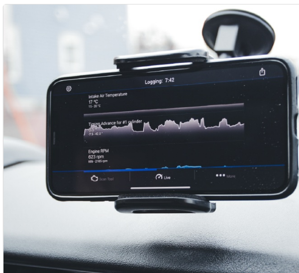
Image: A smartphone screen showing live vehicle data, such as intake air temperature and engine RPM, mounted in a car.
