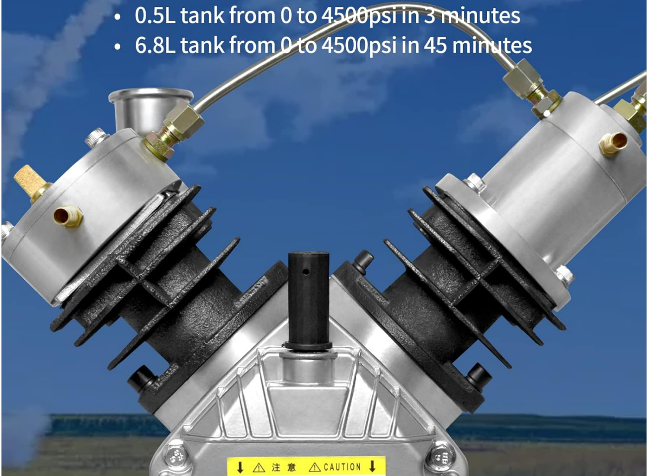
Figure 2.4: Double Cylinder Head with Water Cooling. This close-up shows the double cylinder design, emphasizing the water cooling system. It also provides approximate fill times: 0.5L tank from 0 to 4500psi in 3 minutes, and 6.8L tank from 0 to 4500psi in 45 minutes.
