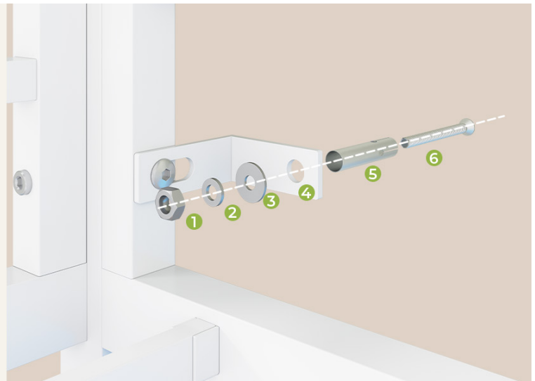
Image: Diagram illustrating the installation of the anti-tipping device for enhanced stability.
