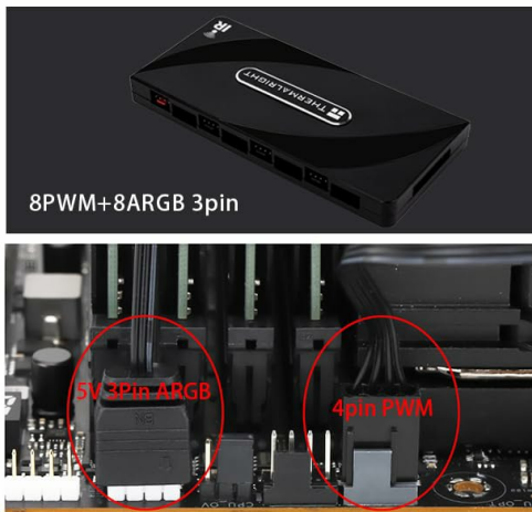
Image 4.2: Diagram showing the SATA direct power input, 8 PWM fan ports, and 8 ARGB 3-pin ports. The red port is highlighted for fan speed recognition.
