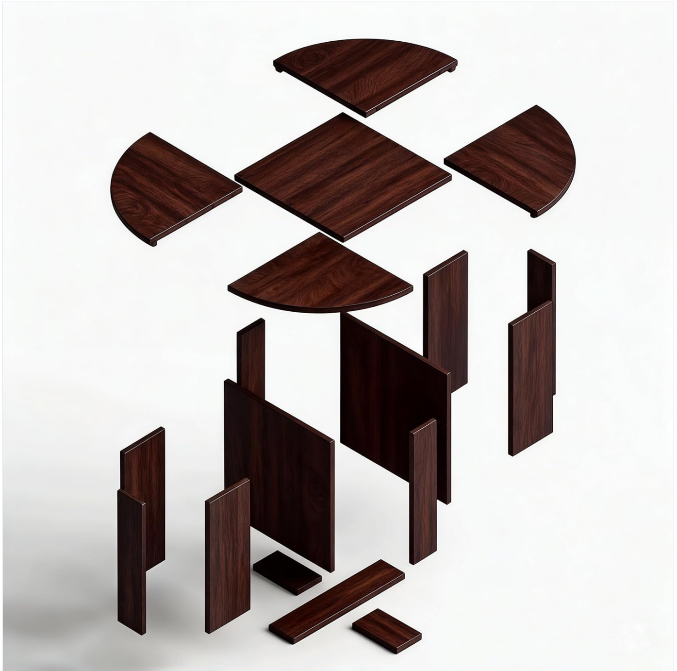
Figure 2: Exploded view of table components
