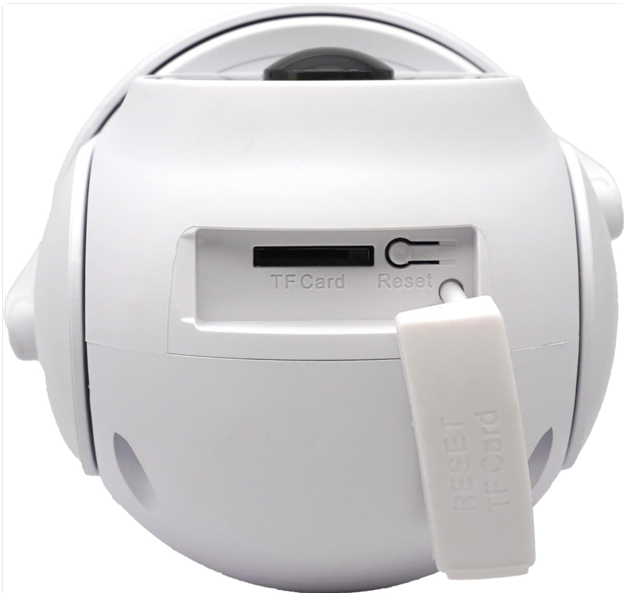
Image 3.1: Location of the TF Card slot and Reset button under the protective cover.
