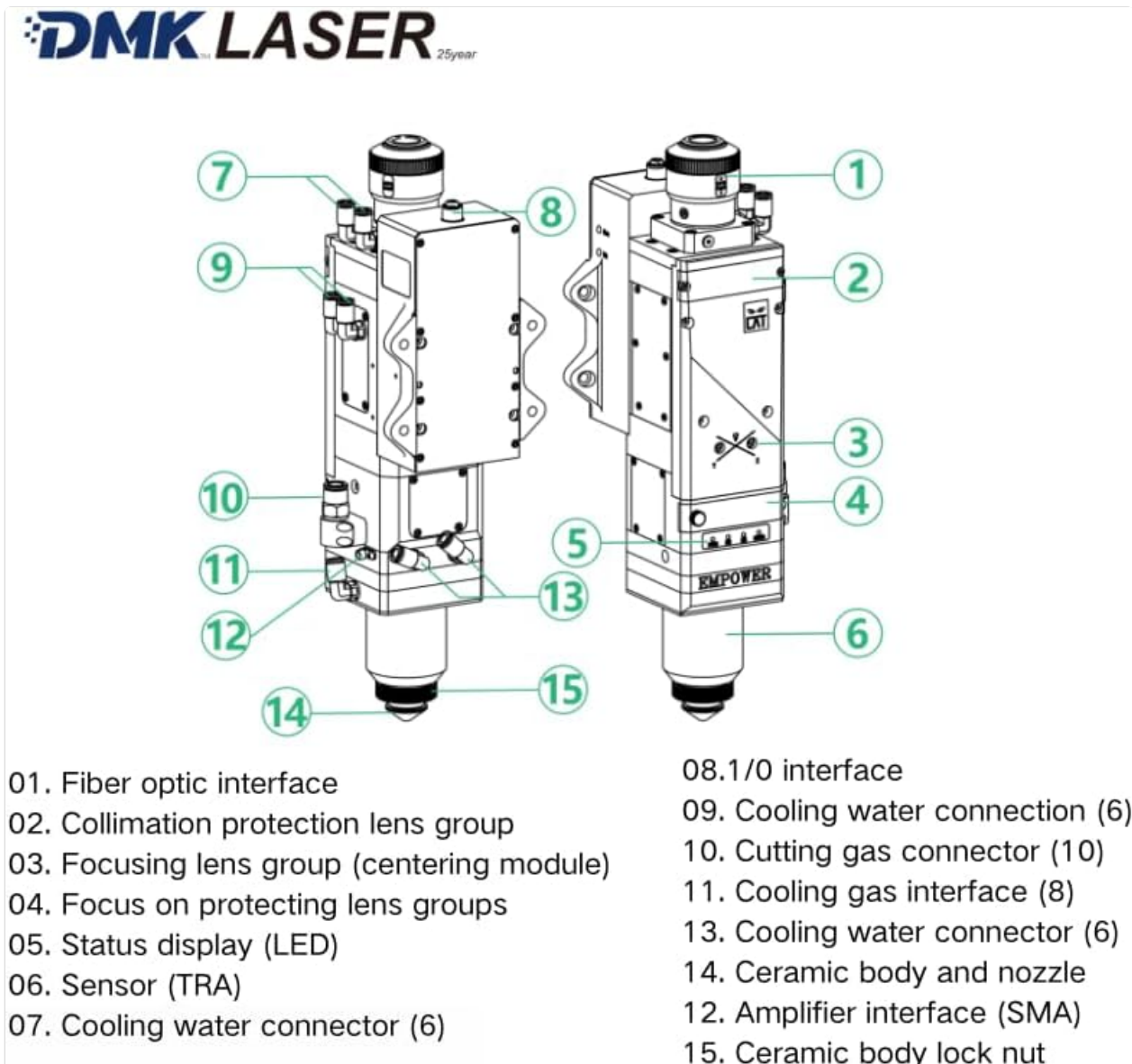
Figure 2: Key components of the BS06K-CAT-2D Laser Cutting Head.
