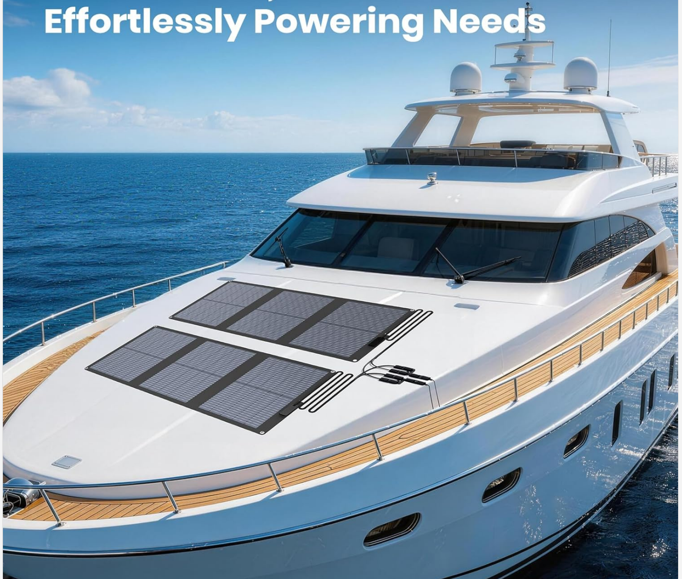
Figure 3: Deployment Example. The two 60W solar panels are shown deployed and connected in parallel on a boat deck, ready to capture sunlight.
