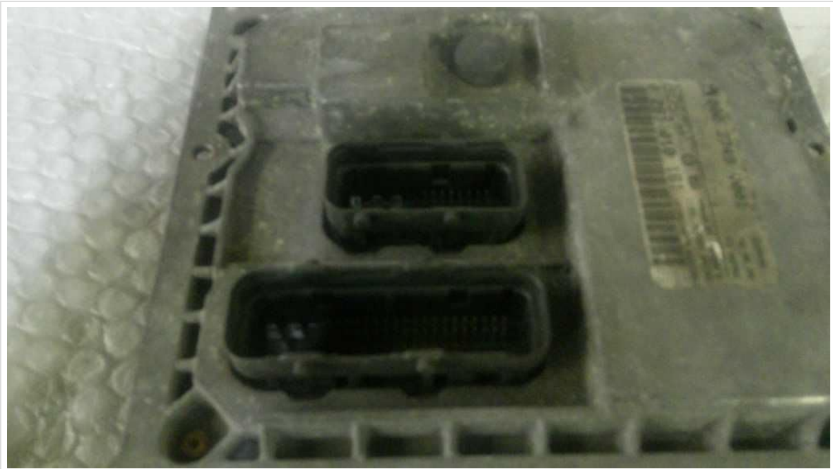
Figure 2: Detail of the ECM's multi-pin electrical connectors, which must be securely attached during installation.
