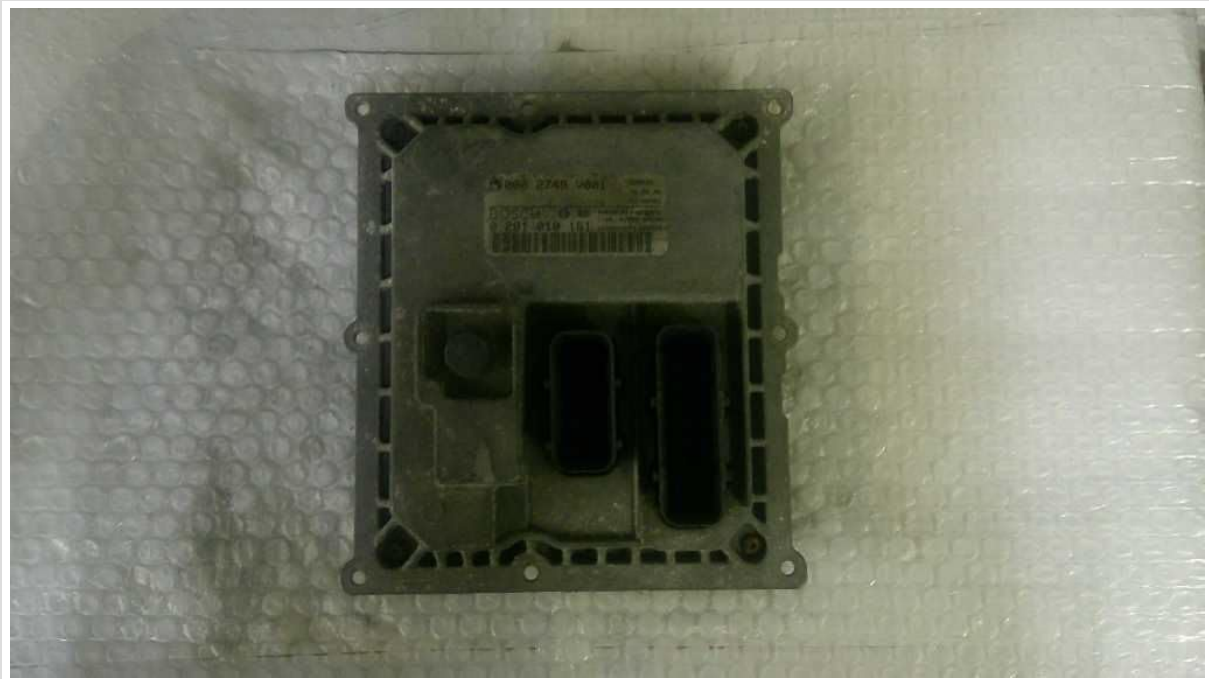
Figure 1: Top view of the Engine ECM Control Module, showing its robust casing and connector ports.
