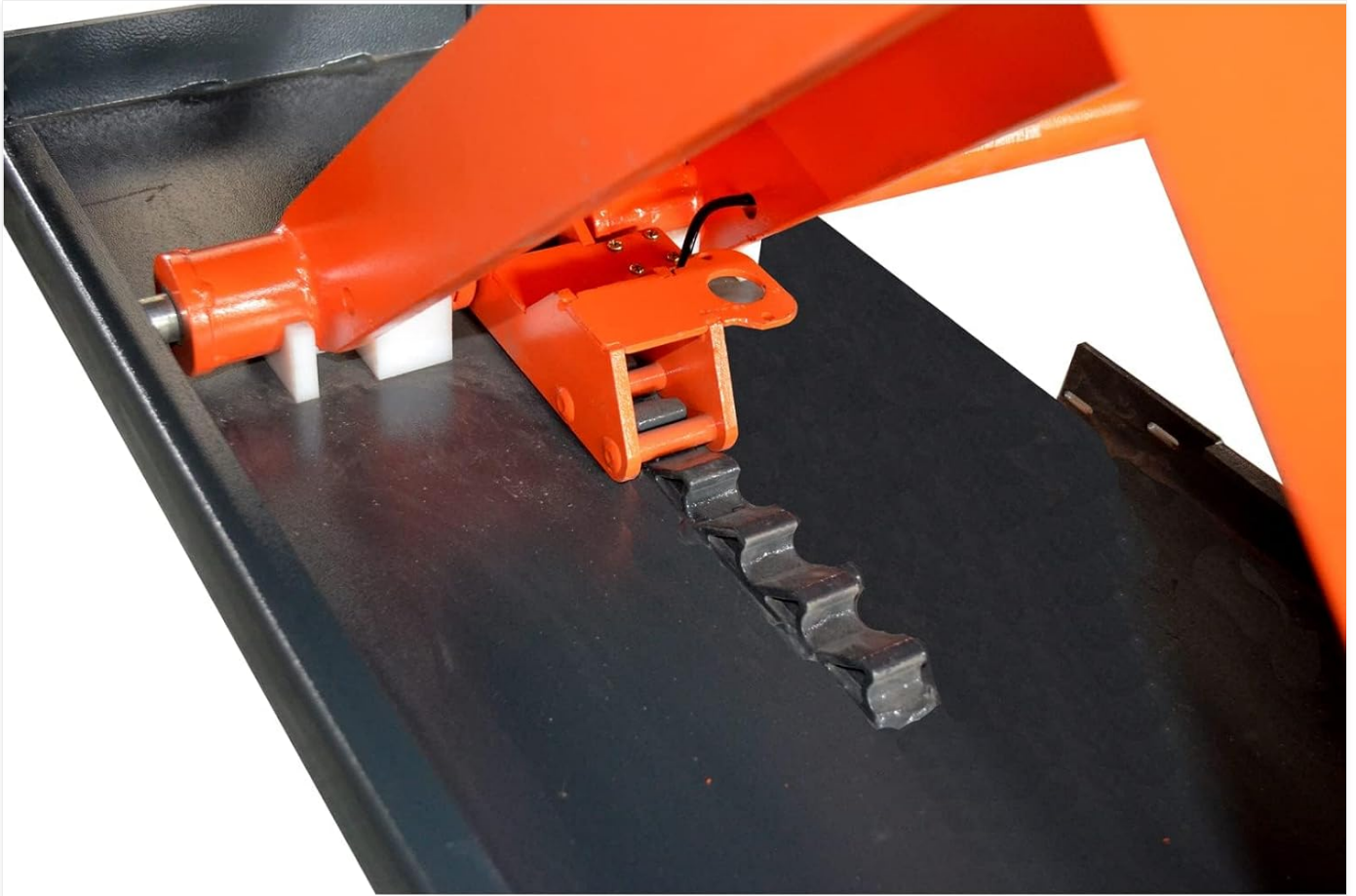
Figure 6: Detail of the safety locking mechanism, crucial for securing the lift at working height.
