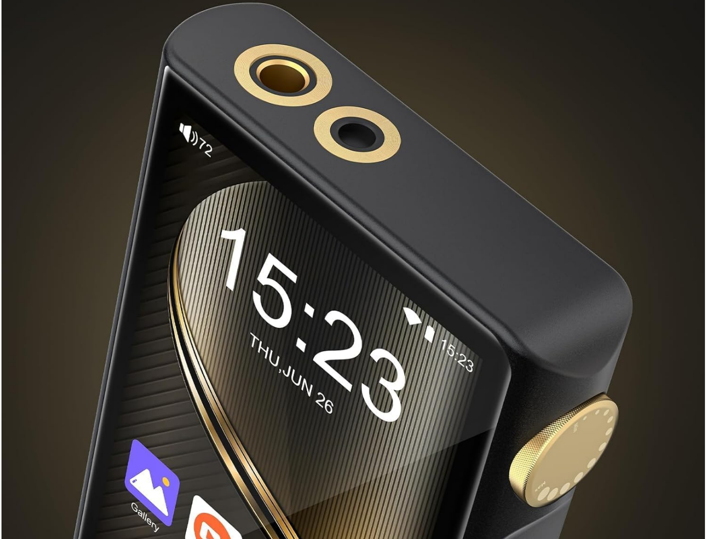
Image: Top view of the ZAQE P30, highlighting the 3.5mm and 4.4mm headphone output jacks.
