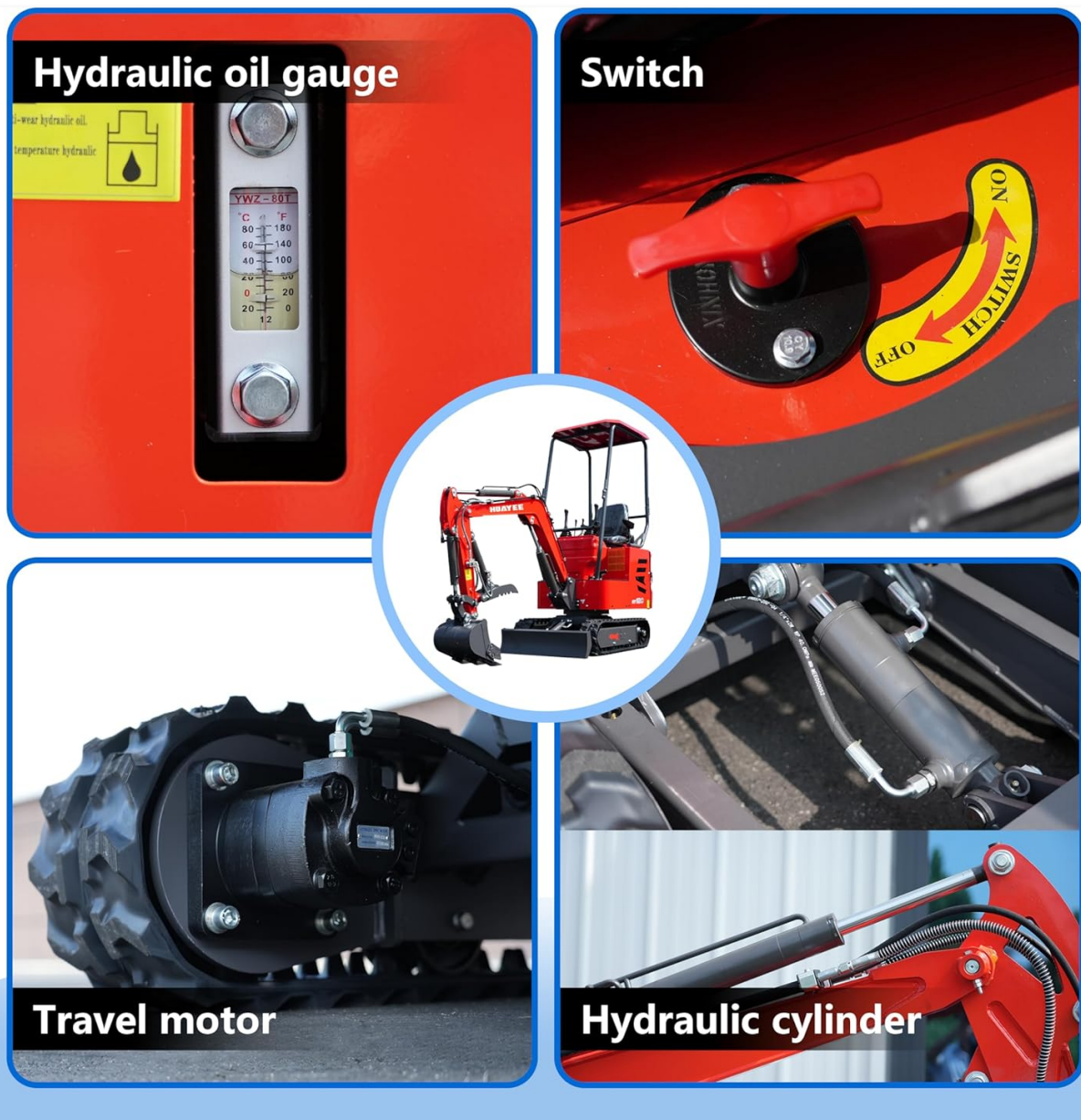
Figure 4: Essential indicators and components including the hydraulic oil gauge, engine switch, travel motor, and hydraulic cylinder.
