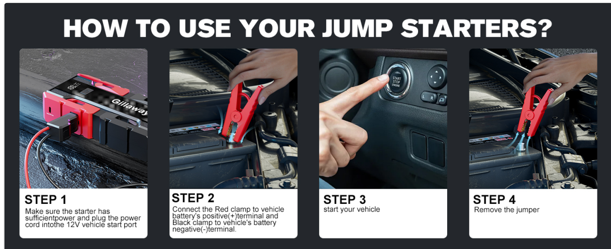
Figure 3: Step-by-step guide for jump starting.
