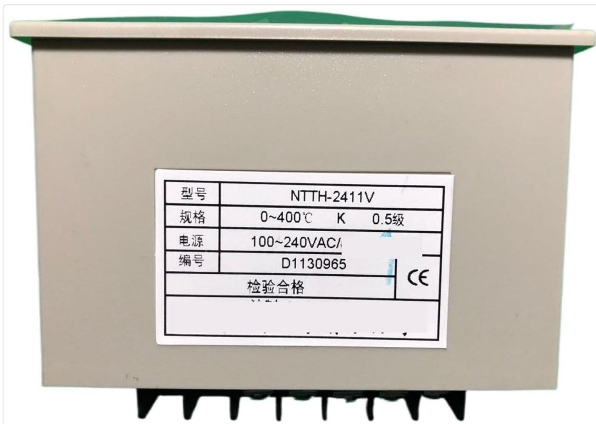
Figure 2: Rear panel label showing model number, temperature range, thermocouple type, power supply, and serial number.
