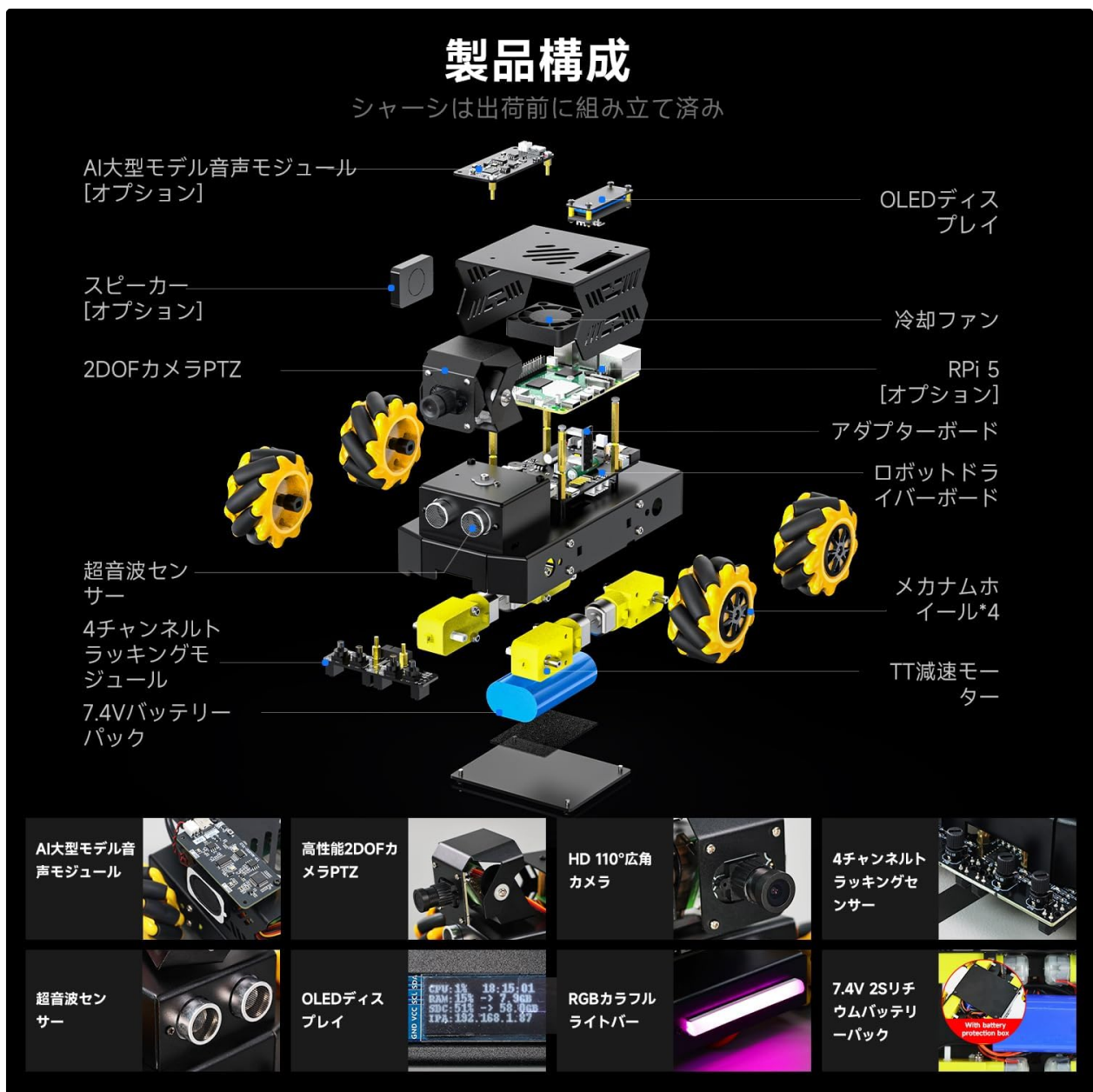
Figure 2: Exploded view illustrating the various components of the Raspbot V2, including the Raspberry Pi 5, camera, sensors, and drive system.
