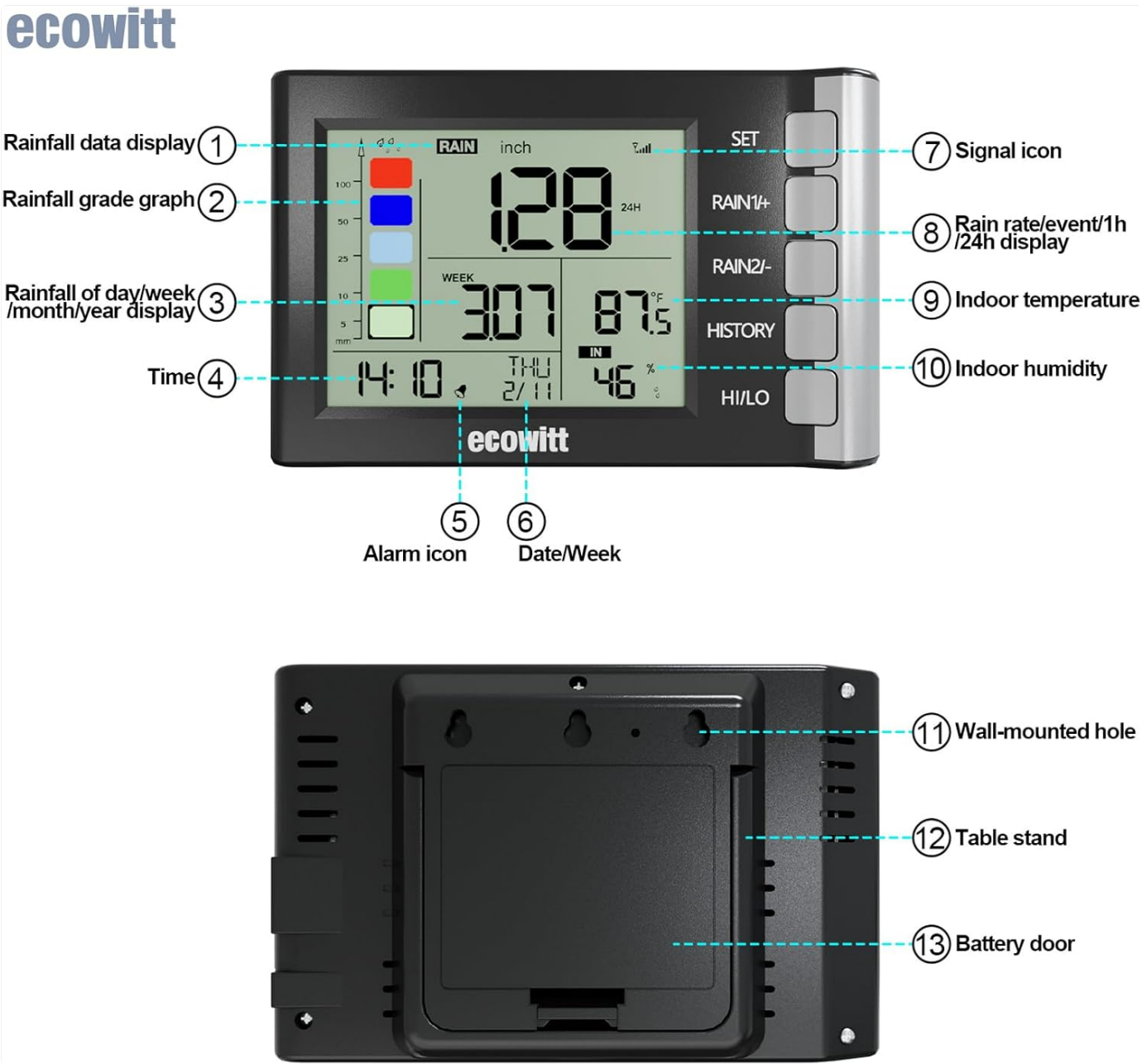
Front view of the WH5370_C Display Console with numbered labels indicating: (1) Rainfall data display, (2) Rainfall grade graph, (3) Rainfall of day/week/month/year display, (4) Time, (5) Alarm icon, (6) Date/Week, (7) Signal icon, (8) Rain rate/event/1h/24h display, (9) Indoor temperature, (10) Indoor humidity. The back view shows: (11) Wall-mounted hole, (12) Table stand, (13) Battery door.
