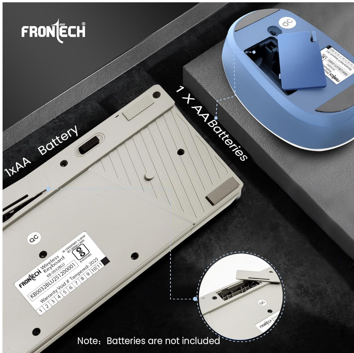
Image 2.1: Battery installation for the keyboard and mouse.
