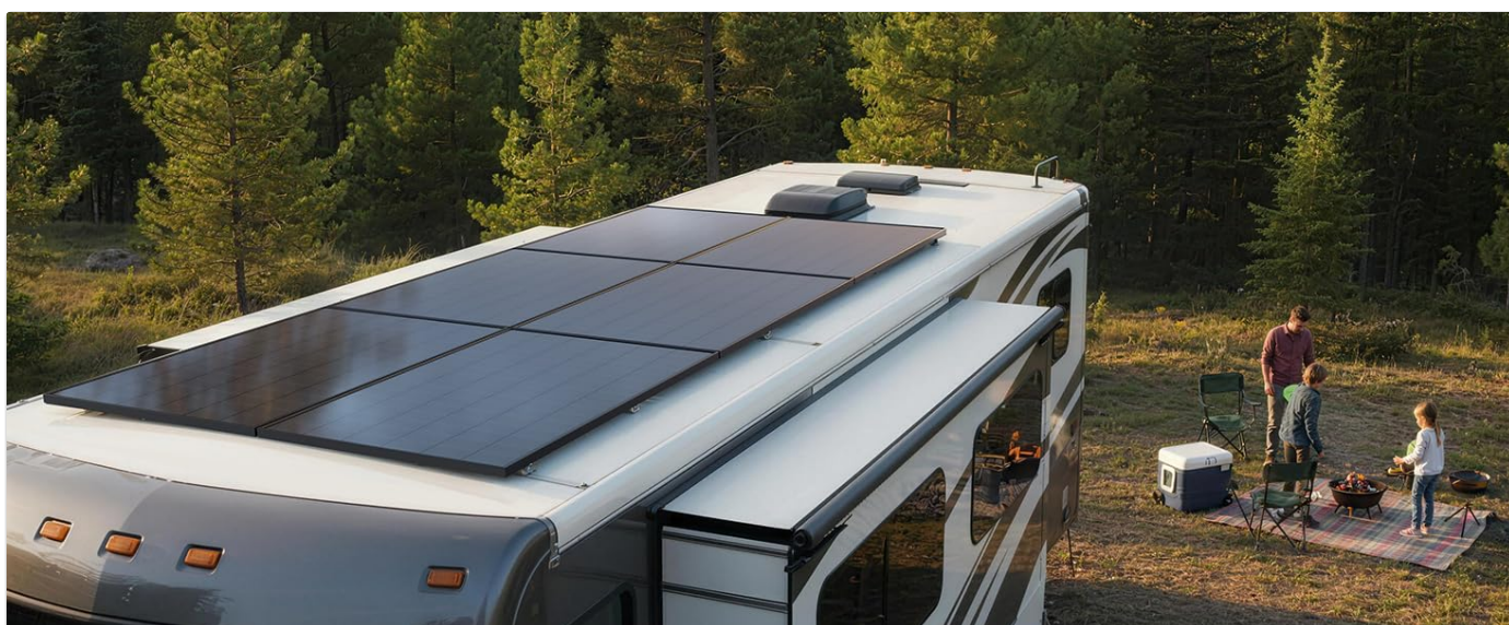
Figure 9: RV installation example.
