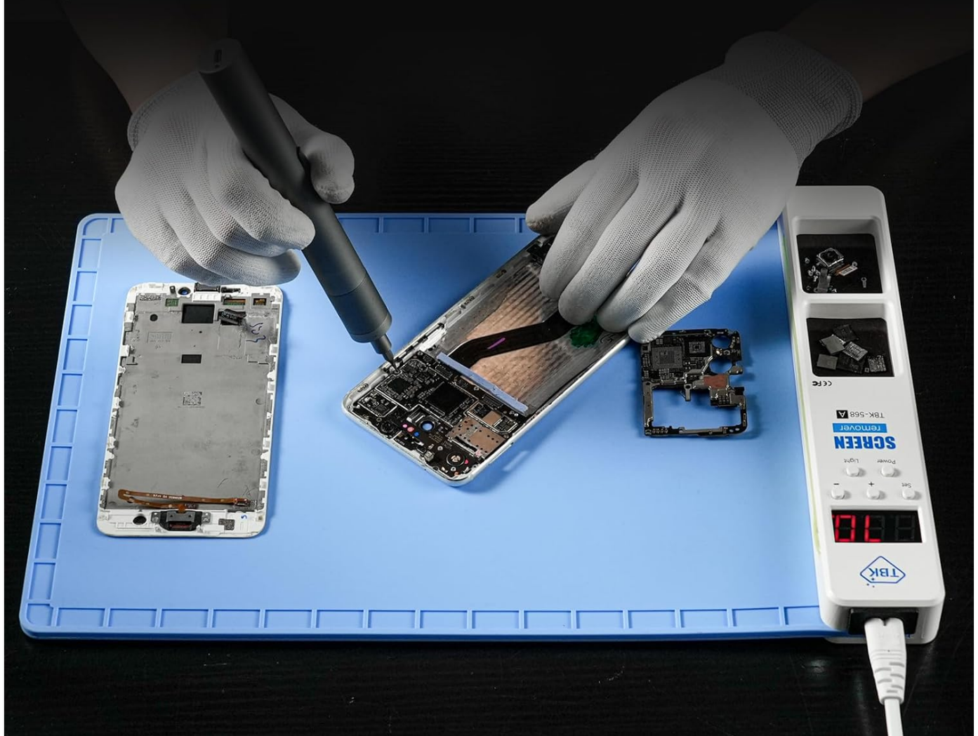
Figure 6: An individual performing a phone repair on the TBK568A Heating Pad, demonstrating its use as a stable and heated work surface.
