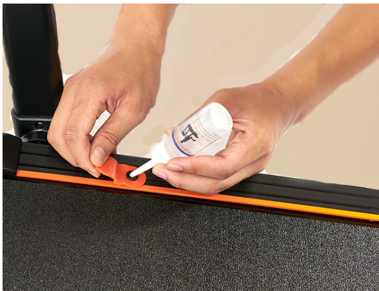
Figure 12: Easy-Self Lubrication. Apply lubricant through the designated hole to maintain the running belt. Run the treadmill for 10 minutes after application for even distribution.
