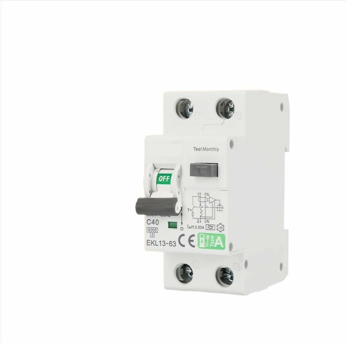
Figure 6.1: The ETEK RCBO EKL13-63 showing the 'Test Monthly' button. Pressing this button simulates an earth leakage fault to verify proper operation.
