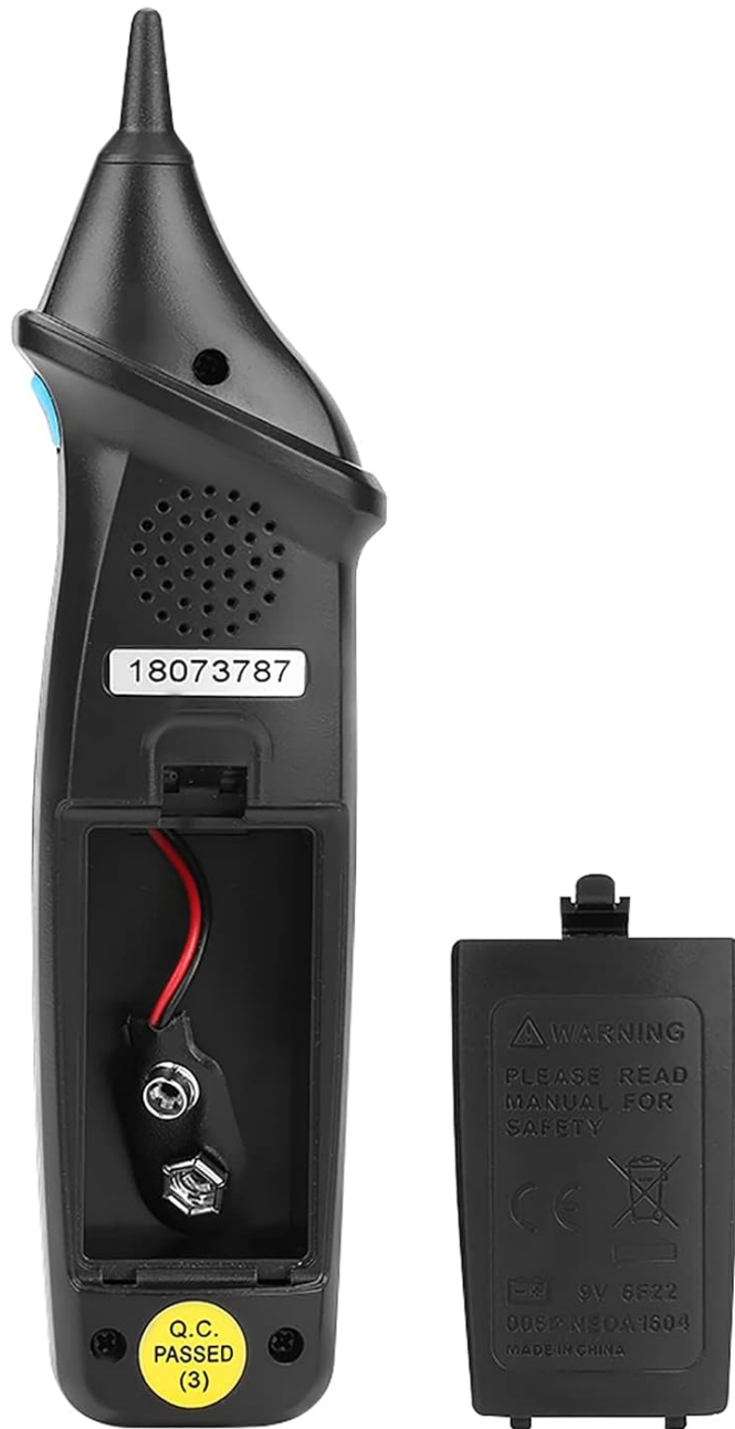
Figure 4.1: The battery compartment of the AVD06 detector, showing where to insert the 9V battery.
