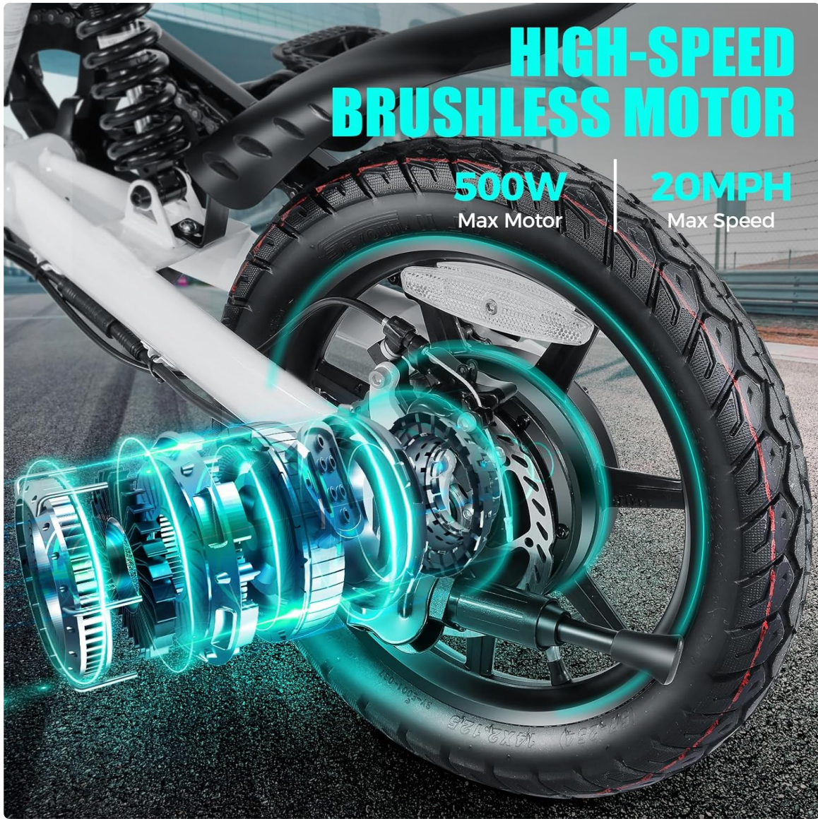
Image: The high-speed brushless motor and disc brake system.
