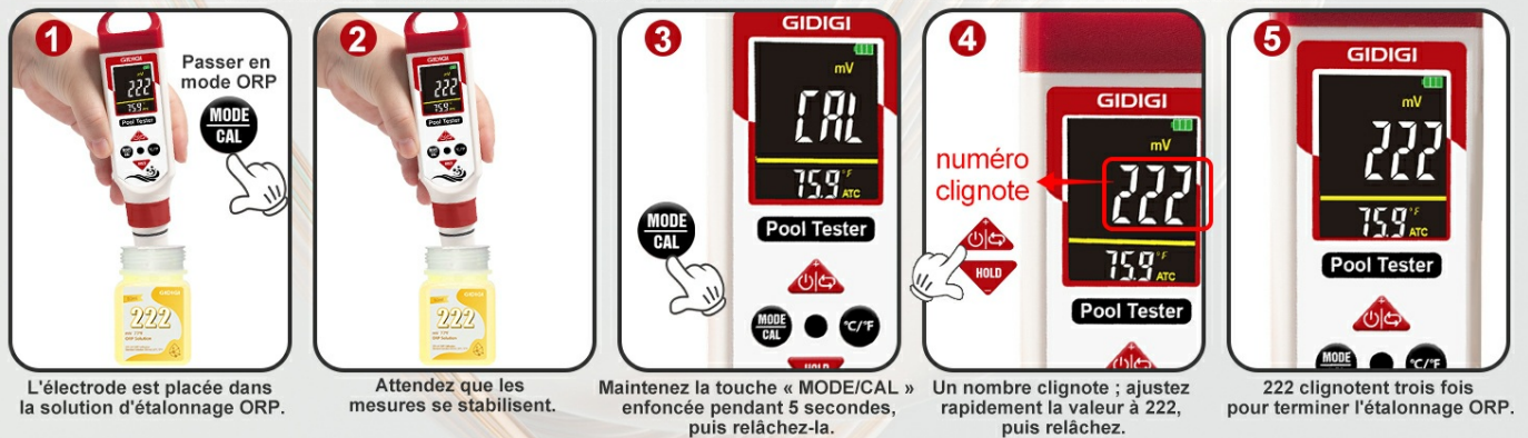
Image 6.3: ORP 222mV Calibration Procedure.
