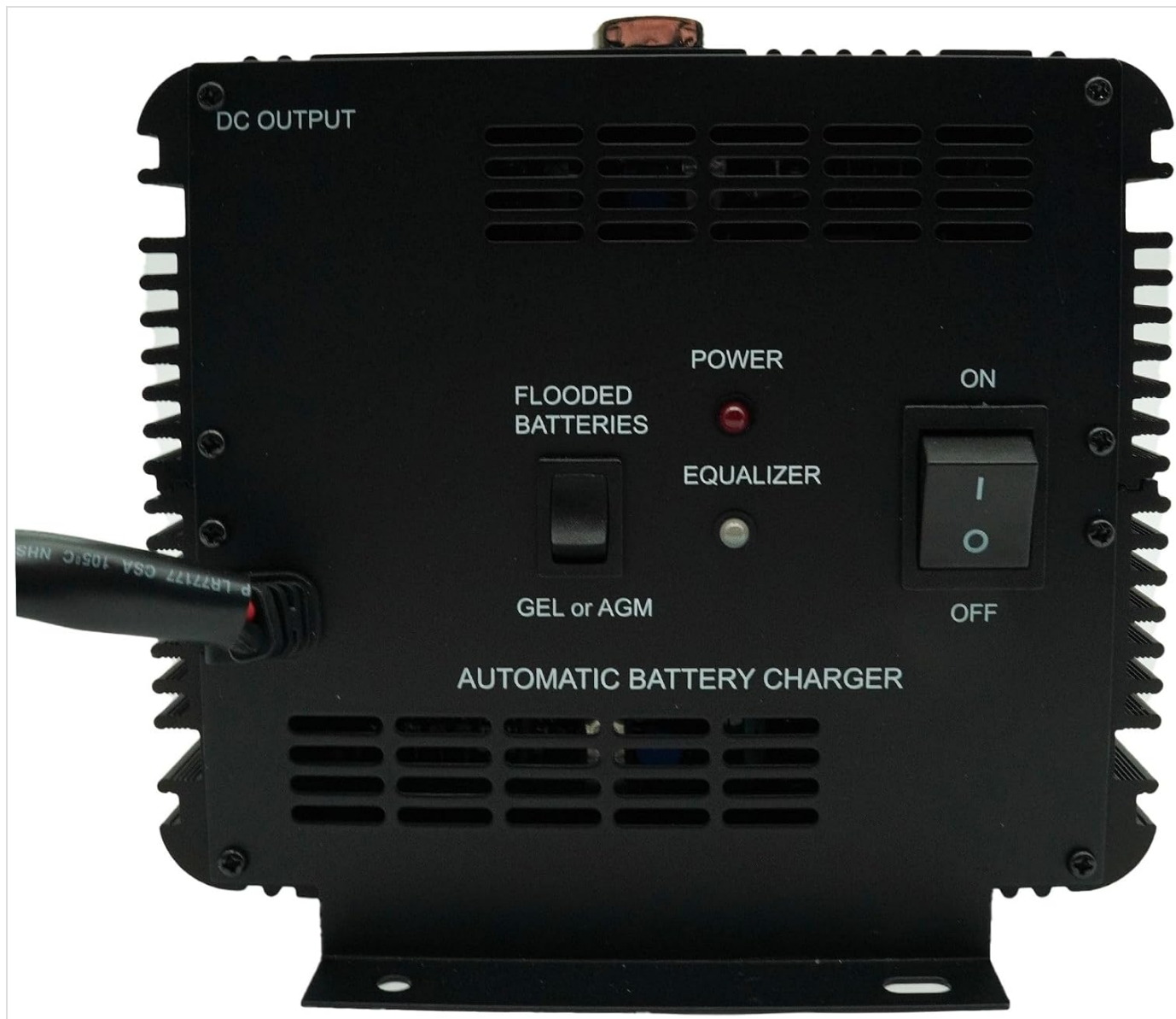
Image 4.1: Front panel of the charger, displaying the DC output, power switch, battery type selector, and LED indicators.
