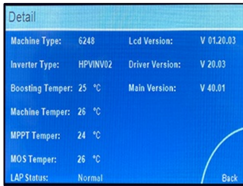
Figure 4.2: LCD screen showing system details including machine type, LCD/driver/main versions, boosting temperature, machine temperature, MPPT temperature, MOS temperature, and LAP status.
