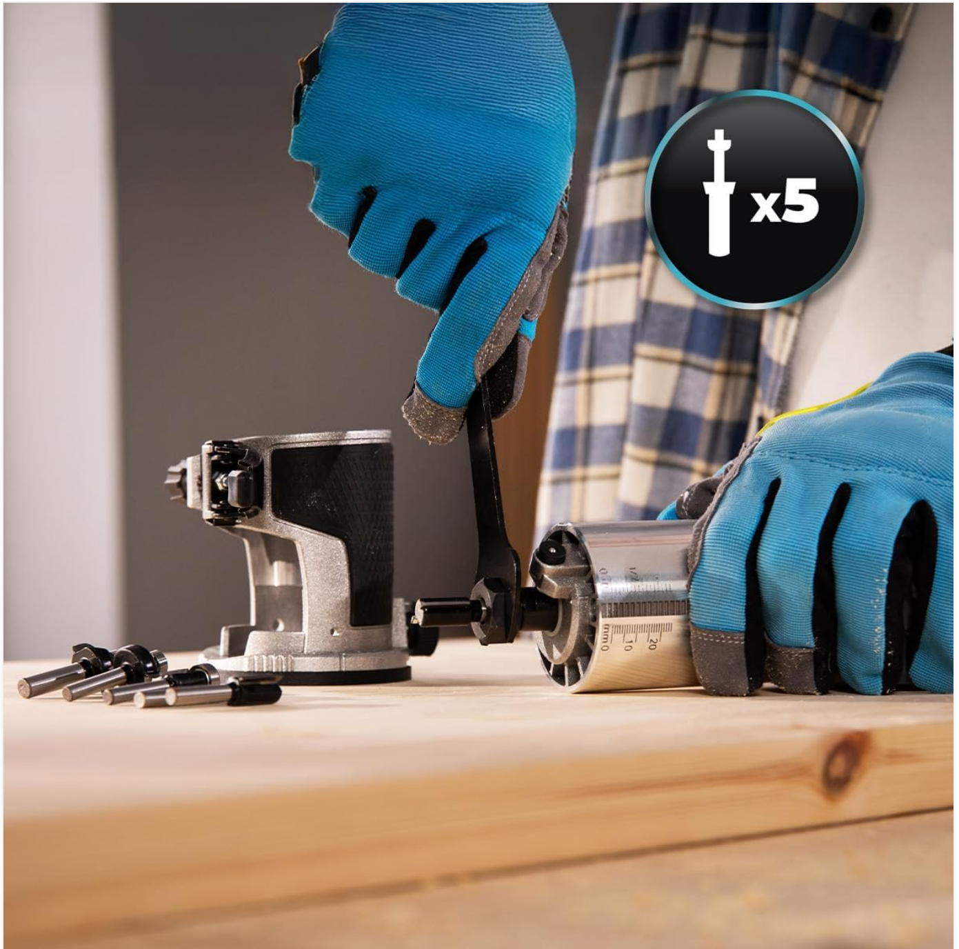
Figure 2: Proper installation of a router bit into the tool's collet.
