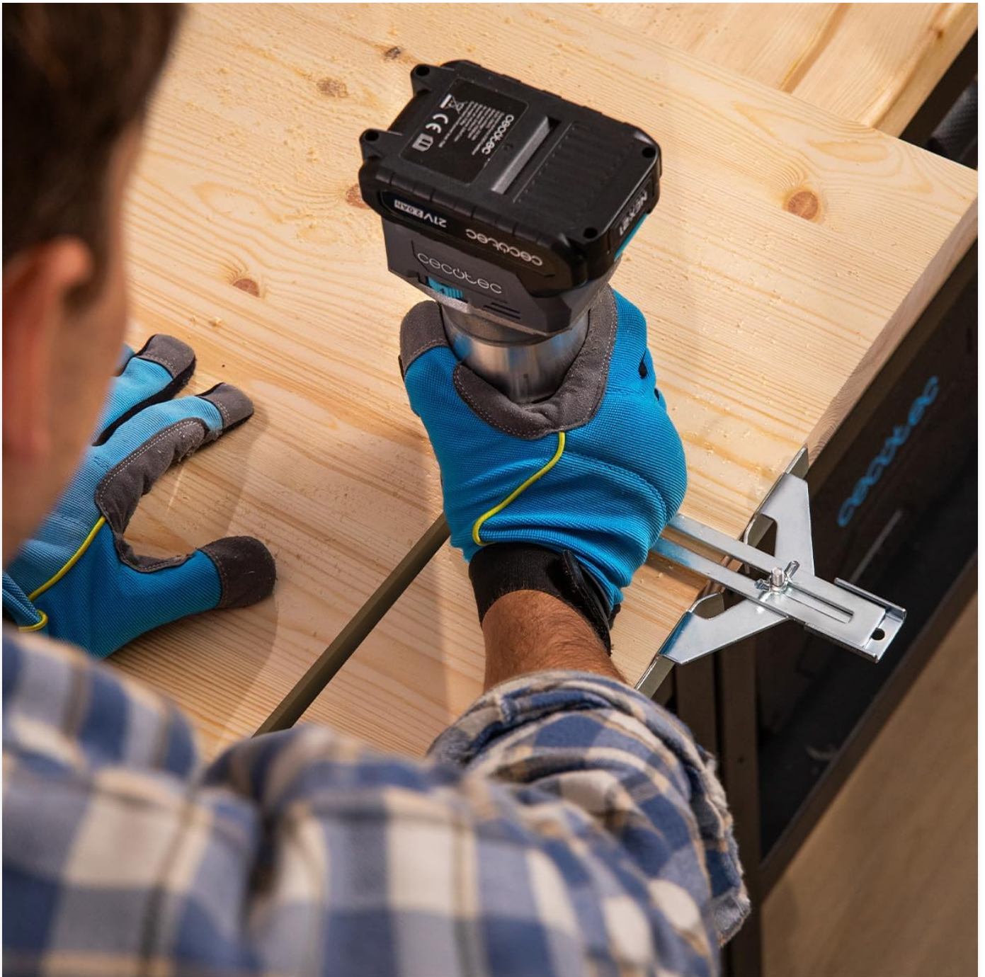
Figure 4: The router in use with the parallel guide for consistent edge routing.
