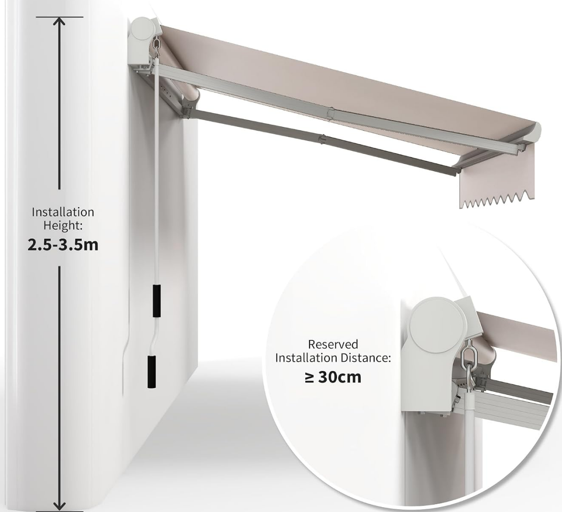
Image 4.1: Recommended installation height and reserved distance.
