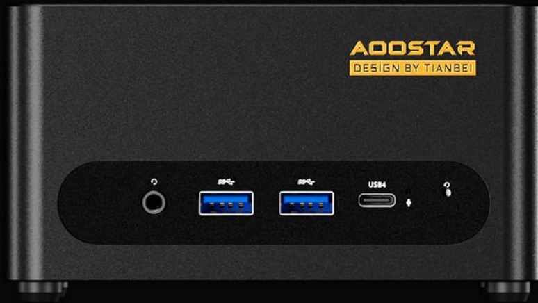
Front Interface Panel: Audio Port ×1, USB3.2 Gen2 ×2, USB4 ×1, Reset Button ×1
