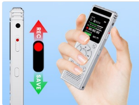
Image: Close-up of the voice recorder showing the 'One Click Recording/Save' switch on the side.
