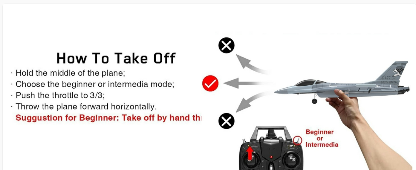
Image: Instructions for hand-launching the RC plane.
