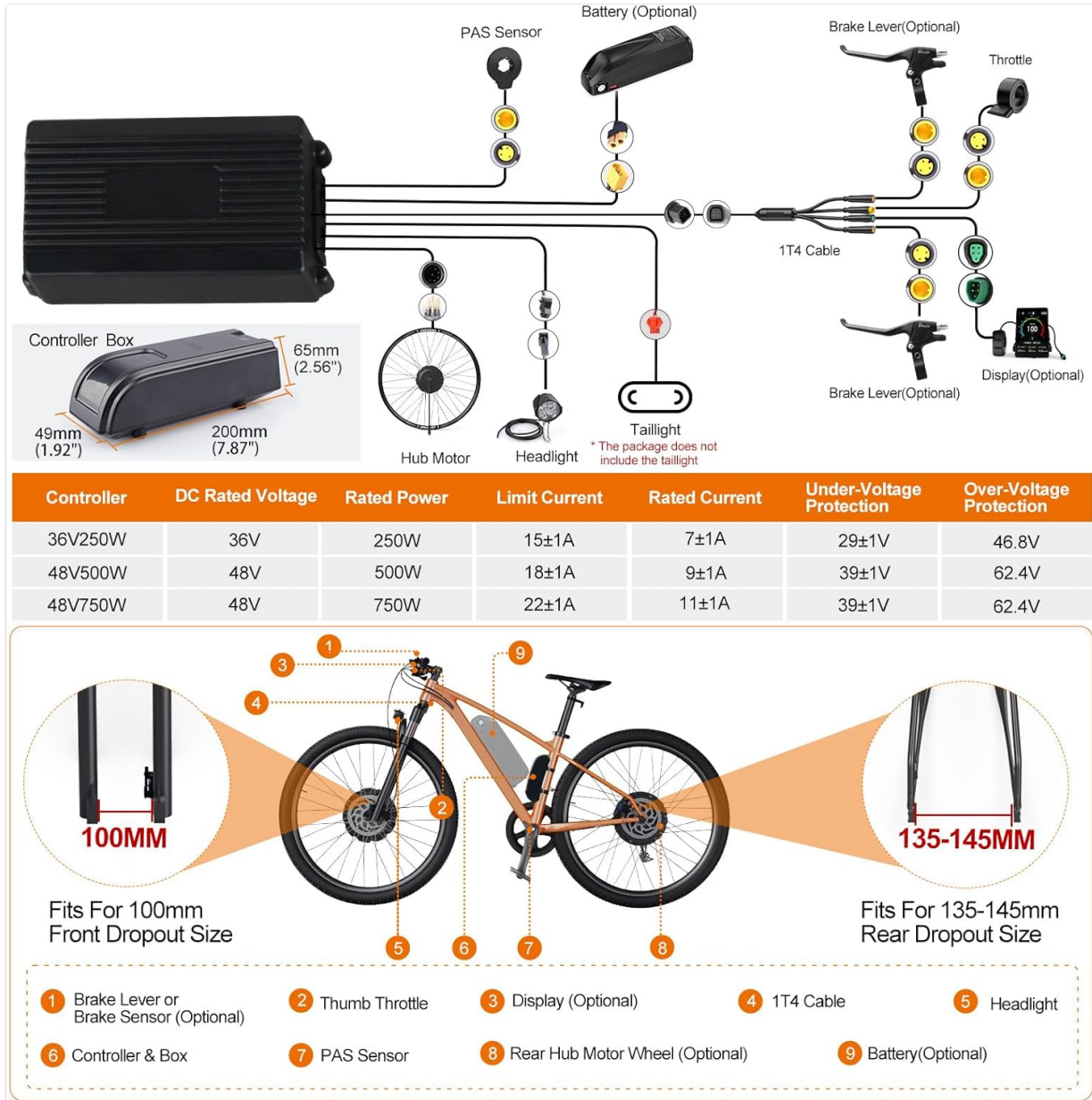
Figure 2.1: Overview of the Varstrom Ebike Conversion Kit components and their connections. This diagram shows the intelligent controller, hub motor, PAS sensor, thumb throttle, brake levers, EKD01 display, headlight, and optional battery, along with a table detailing controller specifications such as DC rated voltage, rated power, limit current, rated current, under-voltage protection, and over-voltage protection.
