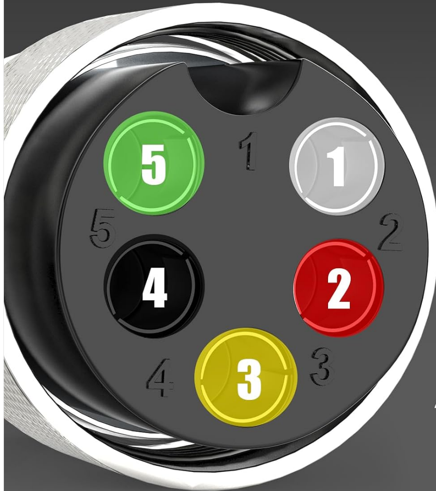
Image 4.2: A detailed view of the 5-pin plug, indicating pins 1, 2, and 4 for amperage adjustment, and pins 3 and 5 for control switch functions.
