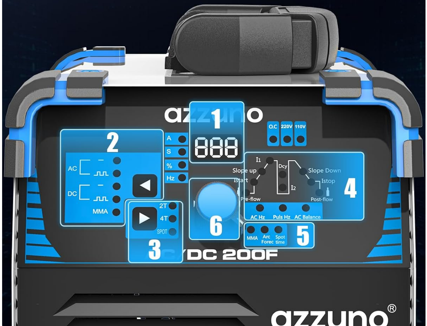
Image 5.1: The control panel of the AZZUNO ACDC-200F, highlighting key areas: 1. Digital Display, 2. Welding Mode, 3. TIG Switch Mode, 4. TIG Parameters Indicators, 5. MMA Function Mode, 6. Knob/Button for adjustments.
