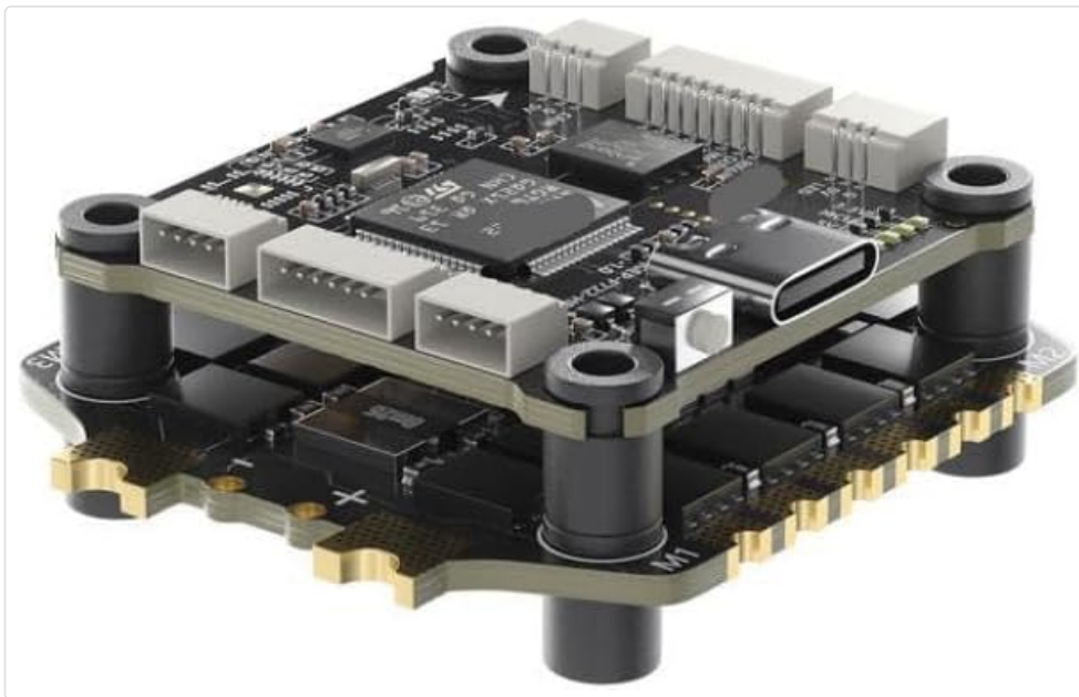
Figure 2.1: Angled view of the assembled flight stack, showing the flight controller and ESC boards.
