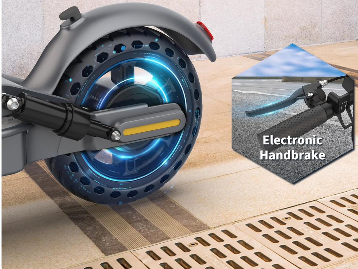
Image: Close-up of the scooter's rear wheel and electronic handbrake, illustrating the dual braking system.
