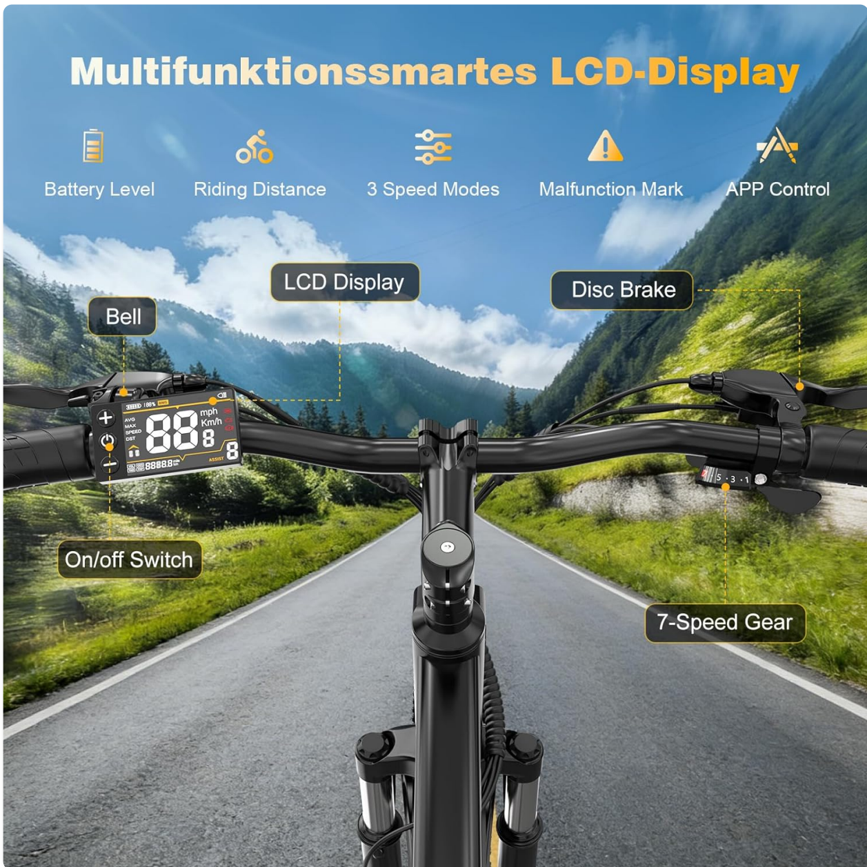
Figure 5.5: Close-up of the multifunctional smart LCD display and handlebar controls, showing battery level, riding distance, speed modes, and other indicators.
