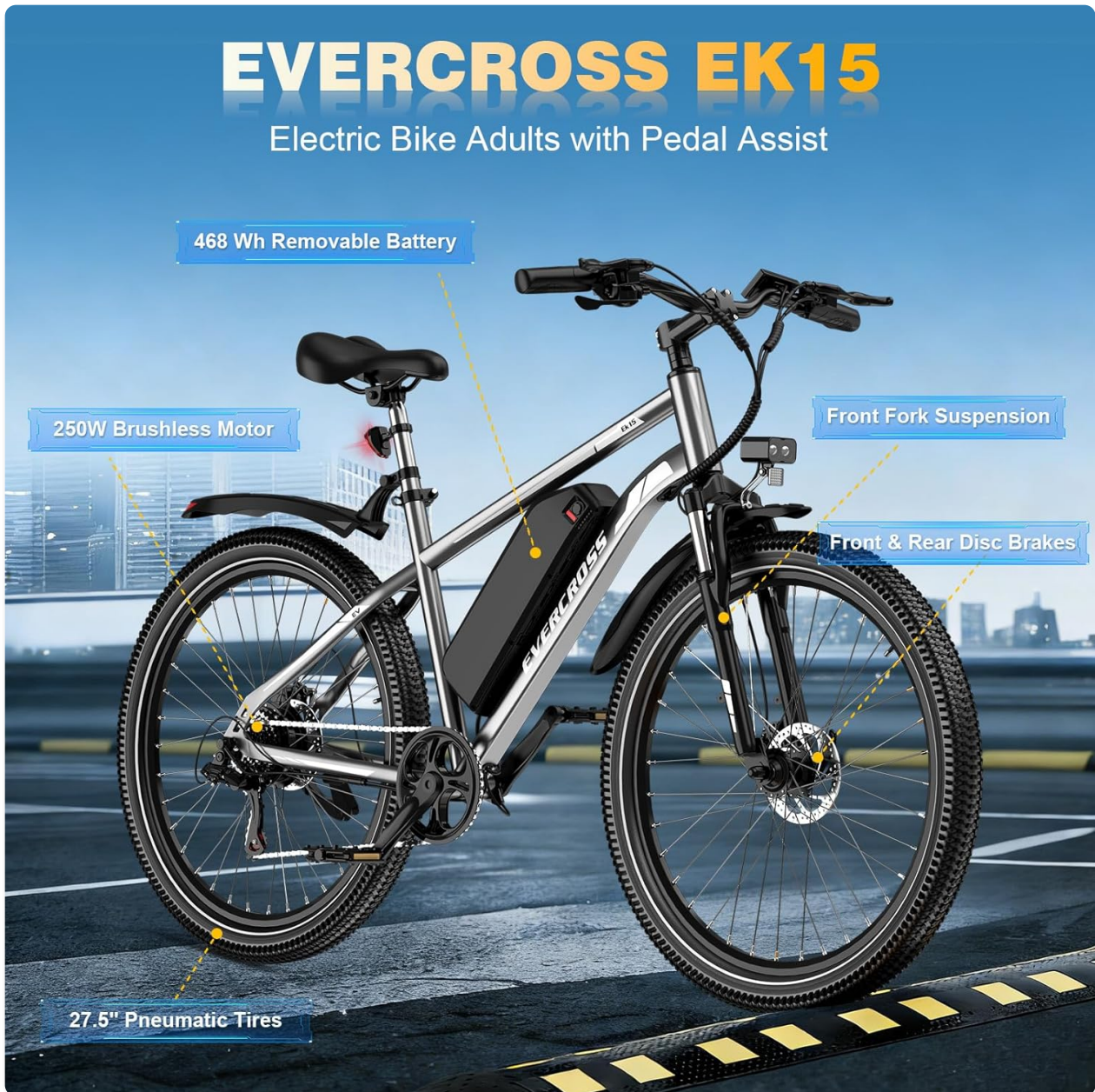
Figure 3.1: Overview of the EVERCROSS EK15 Electric Bike, highlighting key components such as the 250W Brushless Motor, 468 Wh Removable Battery, Front Fork Suspension, Front & Rear Disc Brakes, and 27.5" Pneumatic Tires.
