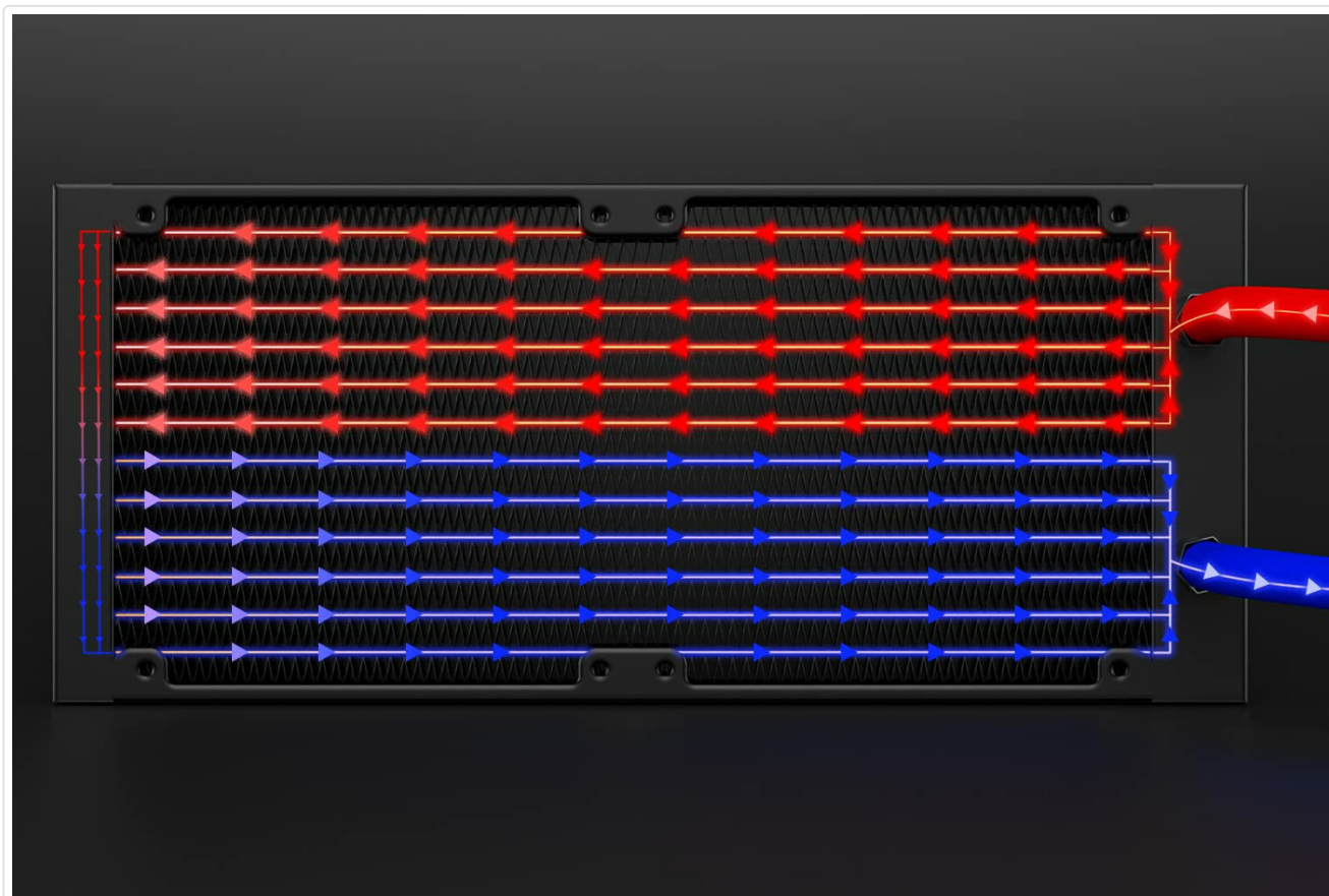
Image: Radiator heat dissipation diagram.
