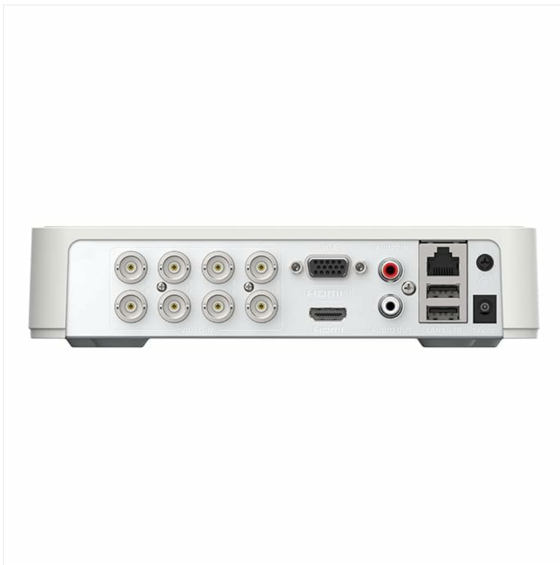
Figure 2: Rear panel of the Hikvision DS-7108HGHI-M1/T DVR. This image illustrates the various connectivity ports available on the back of the device, including multiple BNC connectors for camera inputs, VGA and HDMI outputs for display, audio input and output jacks, an Ethernet port for network connection, USB ports for peripherals, and the DC power input.
