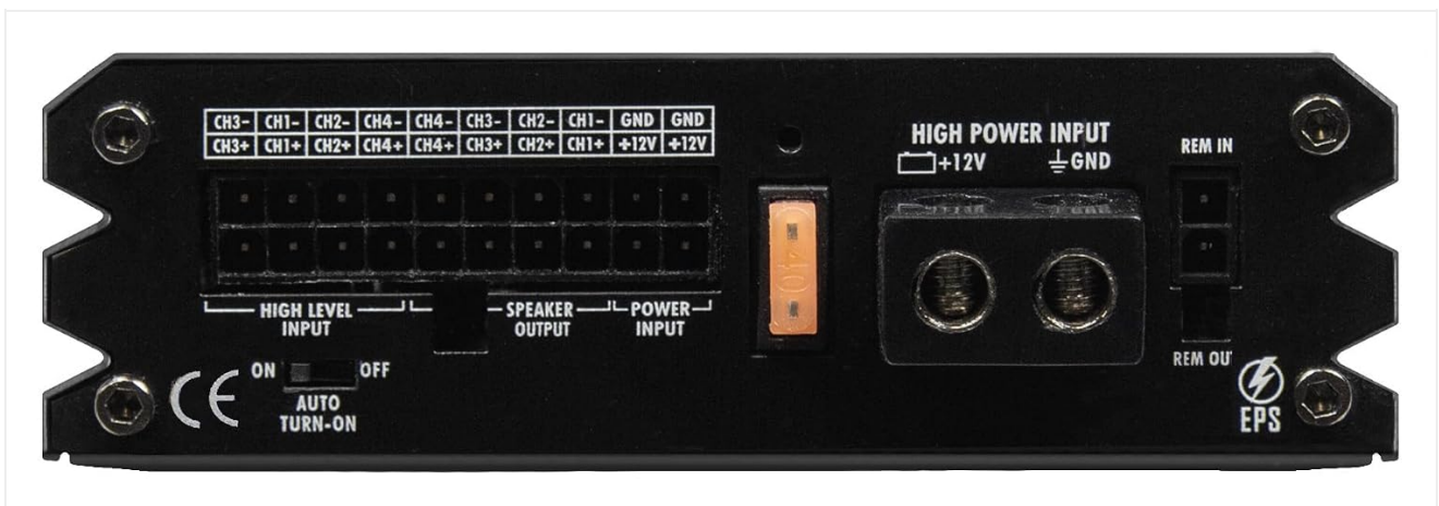
Figure 4.1: View of the front panel of the JUNO4DSP, showing various input and output ports.
