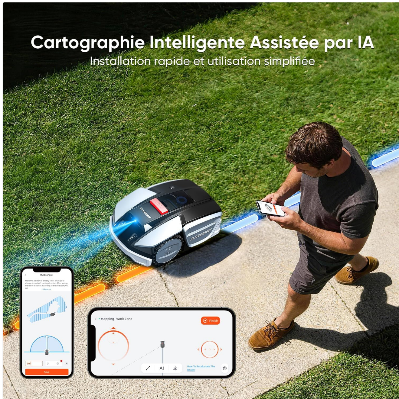
Figure 2.2: AI-Assisted Smart Mapping. The image illustrates the mobile application interface for mapping the garden, showing how the robot mower creates a digital map without physical boundary wires.
